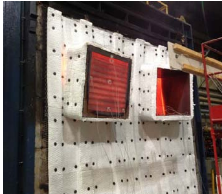
Hydrocarbon Fire Test for a Duplex ST in a H60 Steel Bulkhead
