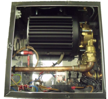
Pump Motor Compartment
